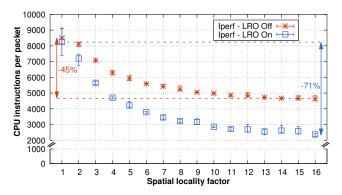
Figure 2: Impact of packet spatial locality on CPU instructions per packet of an iperf server, with or without LRO.
