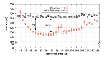
Figure 21: Latency of Reframer when offloaded into a Smart NIC which precedes the NF chain.
