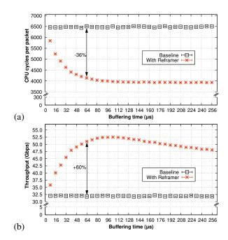
Figure 15: Impacts of Reframer when collocated with the NF chain: (a) Cycles per packet and (b) Throughput.
