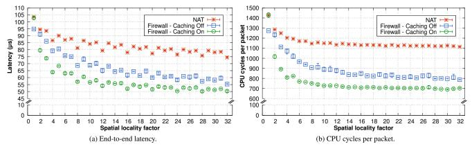
Figure 4: Impact of traffic spatial locality on the packet processing latency and the CPU cycles per packet performance of a NAT and a firewall (with and without rule caching) NFs.
