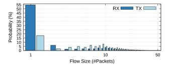
Figure 6: TCP flow size distr. of the analyzed trace with a log. x-axis. The RX trace has  $\sim$  4M flows; the min., avg., and max. flow sizes (in #packets) are 1, 63, and  $\sim$  29M, resp. The TX trace is composed of  $\sim$  2M flows; the min., avg., and max. flow sizes (in #packets) are 1, 137, and  $\sim$  68M, resp.
