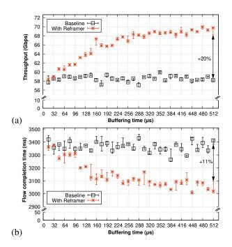
Figure 19: Impact of Reframer when reordering packets of HTTP flows: (a) Throughput and (b) FCT.
