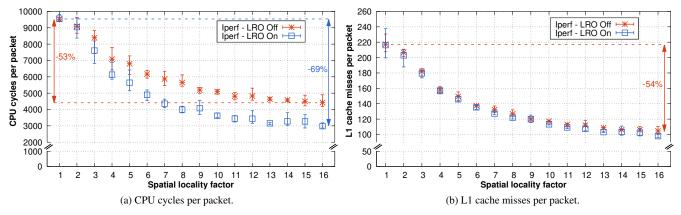
Figure 1: Impact of packet spatial locality on the performance of an iperf server, with and without LRO.
